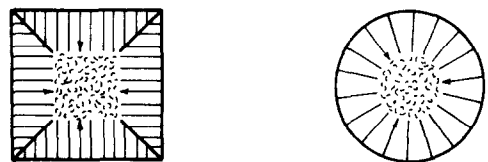
FIG. 1. Natural convection local heat flux density distribution for surface at different positive inclinations in air. (Hot surface, \theta = 38.2 deg. C [6].)
